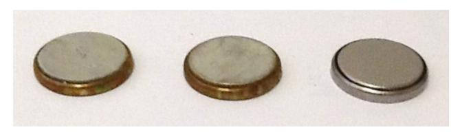
Cell A (left) and cell B (centre) were immersed in boiling water. The cell on the right was new and unused
