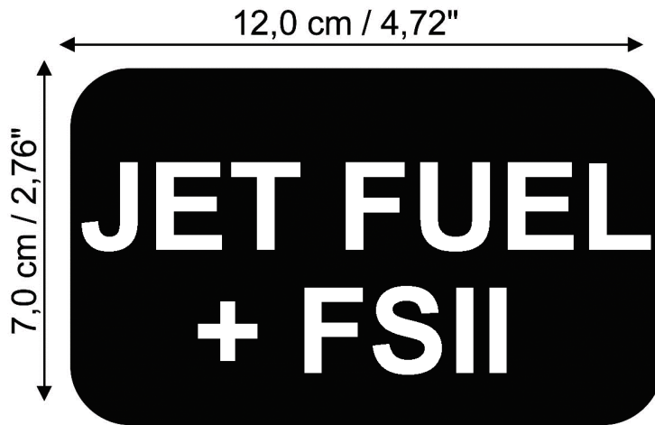
Figure D.5: Decal to be used on aircraft approved to use jet fuel with the mandatory addition of FSII
