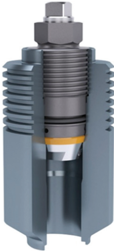
Figure 1: Drawing of a mechanical access fitting configuration. A solid plug assembly is threaded into a weldable access fitting body. Drawing courtesy of Cosasco®
