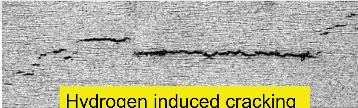
Hydrogen induced cracking
