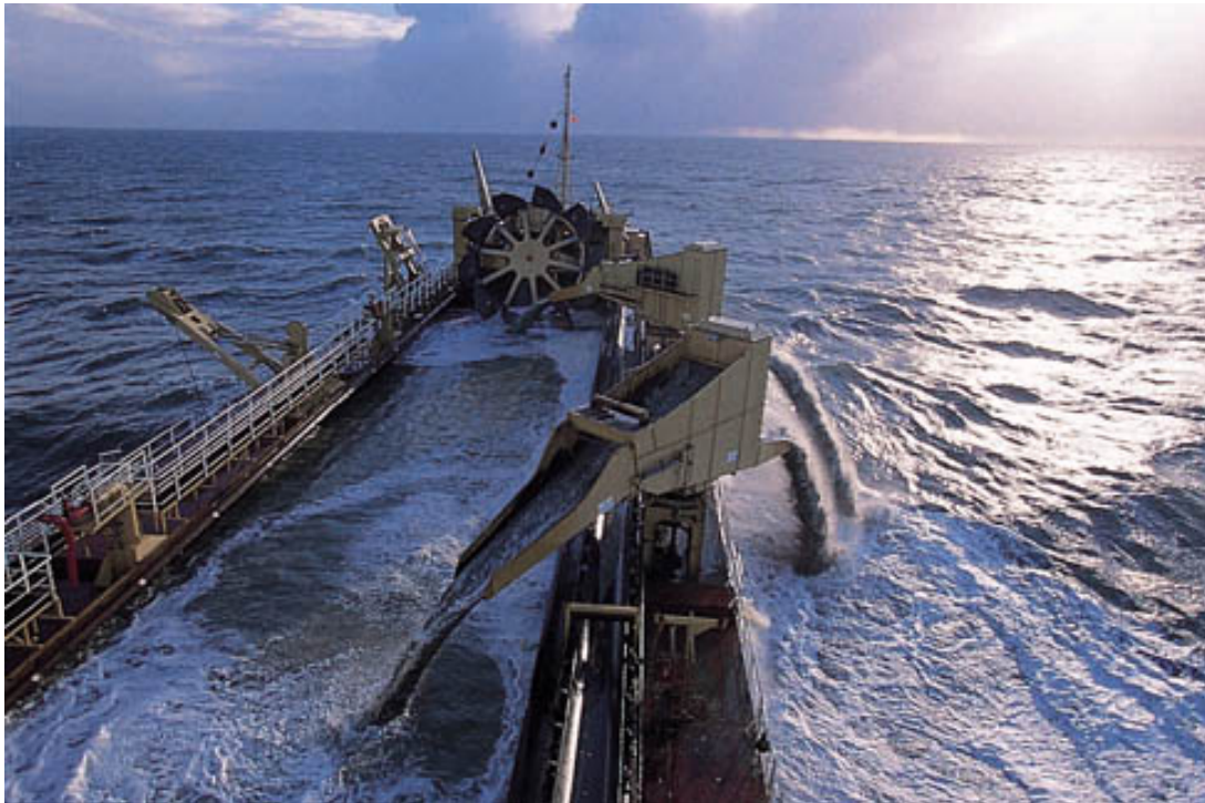
Figure 5.1 Vessel Engaged in Dredging and Displaying RAM Day Marks
