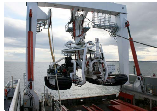
Figure 2-10 i-Trencher chain trenching vehicle & LARS
