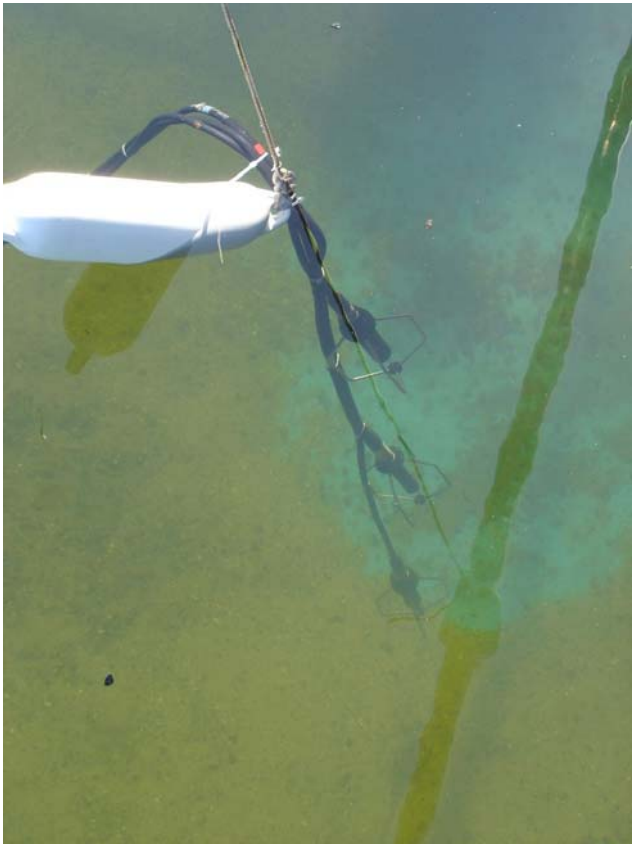
FIG. 26. The 3 B&K 81010 hydrophones used to measure the SPL distribution, suspended at 0.5 m, 1 m, and 1.5 m depth.
