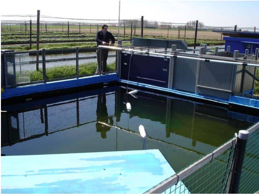
FIG.25. Measurement of the SPL distribution in the harbour seal pool. Note the 1 m markings on the aluminium pole. The white floats support the cables of the 3 hydrophones.
