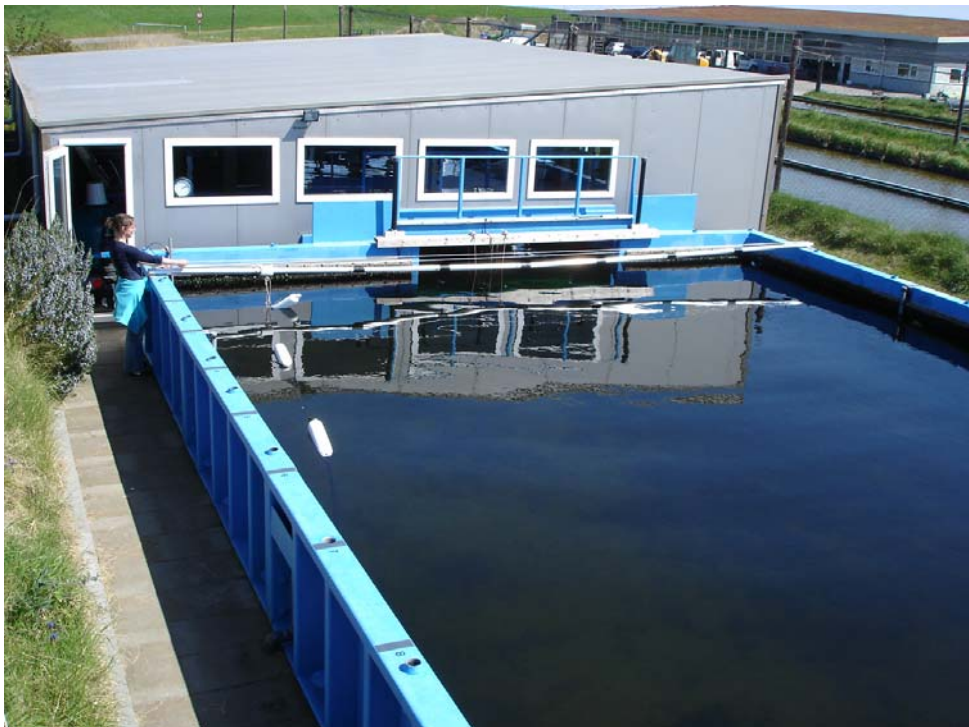
FIG. 12. Measurement of the SPL distribution in the porpoise pool used for the AMD behavioural response study. Note the 1 m markers along the pool sides and on the aluminium pole. Via a pulley system the 3 hydrophones (0.5, 1, and 1.5 m deep) could be pulled along the pole.
