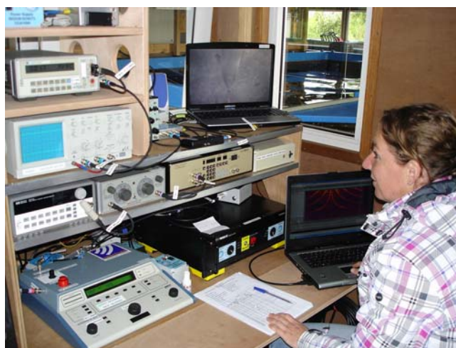
FIG. 6. The signal operator and equipment used for the harbour porpoise AMD audibility study. Note the porpoise in the correct position at the listening station on the screen of a laptop (top), and the spectrum of one of the 3 AquaMark 100 sounds on the screen of a second laptop (bottom right).
