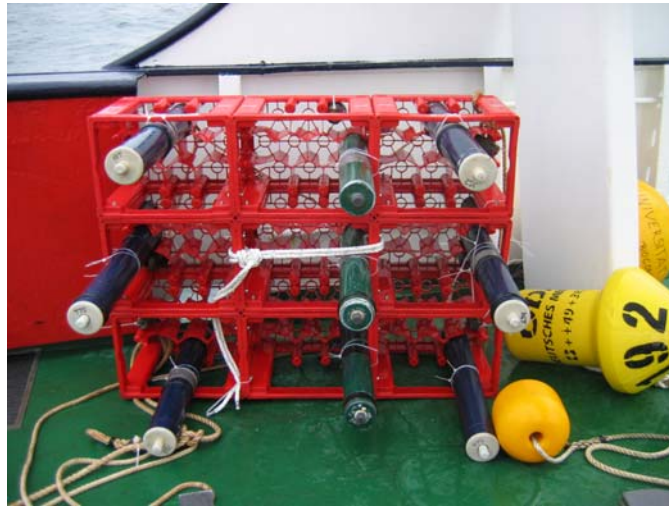
Figure 6-12: Intracalibration of T-PODs close to the wind farm Nysted, from Verfuß et al. (2007c), the devices are separated by at least 30 cm to prevent a bias from interferences and echoes.
