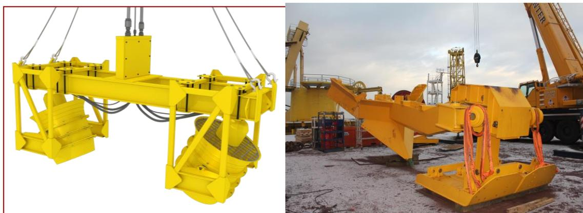
Figure 8: (left) typical mass excavator, most commonly used for cable recovery. Image courtesy of X-subsea; (right) pre-cutting plough that can be used for boulder removal. Image courtesy of Ecosse Subsea Systems.
