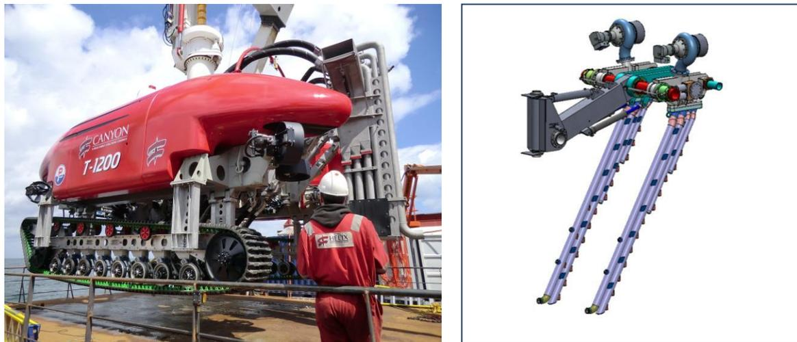
Figure 6: (left) large jet trencher; (right) multi-nozzle jet legs, which are configured and sized relative to the soils to be jetted. Both images courtesy of Helix Canyon Offshore.
