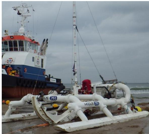
**Figure 5: Typical jet sledge deployed from the beach and used to trench in sands and soft clays. Image courtesy of MODUS Seabed Intervention Limited.**
