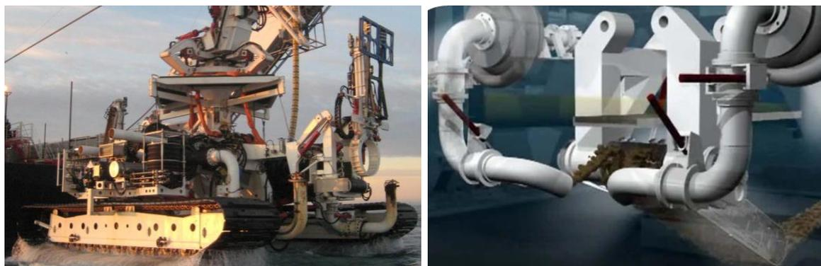
Figure 7: (left) typical hard ground mechanical trencher, which needs to be heavy (normally more than 40t in water); (right) trench being formed by the cutting chain. Both images courtesy of Helix Canyon Offshore.
