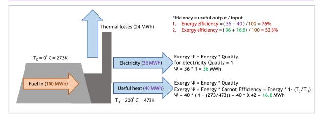
14.52 **Exergy of various power plant types** Assuming all plants have 100 units energy input and the varying quantities of heat and electricity lead to different efficiency in exergy. The most energy efficient plant (boiler) has the highest global warming potential per unit of exergy. *Source: Adapted from Schuller et al.*<sup>649</sup>
