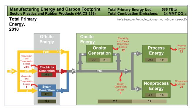
14.4 **US plastics energy and carbon flow** The energy flows are indicated by the arrows and the indirect and direct carbon emissions are shown in the brown boxes below each step. The flows in these steps are then broken down further in a second illustration (not shown here). Source: US Department of Energy.<sup>220</sup> Don't automatically assume the **largest users of resource** offer the greatest savings potential.
