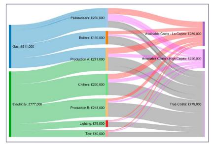
16.21 Sankey diagram illustrating the savings potential for electricity and gas in various departments in a small dairy Source: Niall Enright. Based on real client data. Drawn using SankeyMATIC.
