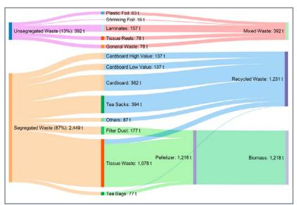
16.20 Sankey diagram illustrating the proposed flow of solid wastes in a tea bag manufacturer Source: Niall Enright. Based on real client data. Drawn using SankeyMATIC. Broadly speaking, I would divide Sankey software into two general types.
