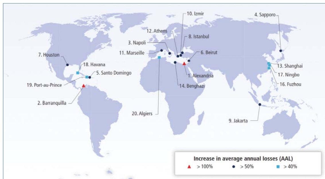
Figure 6. The 20 coastal cities where average annual losses (AALs) increase most (in relative terms in 2050 compared with 2005) in the case of optimistic sea level rise, if adaptation maintains only current defence standards or flood probability (PD)
