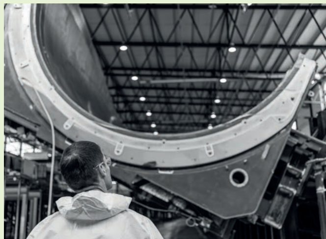
Blade construction at West Medina Mills – showing a cross section of one half of a V164 blade Photo: MHI Vestas Offshore Wind
