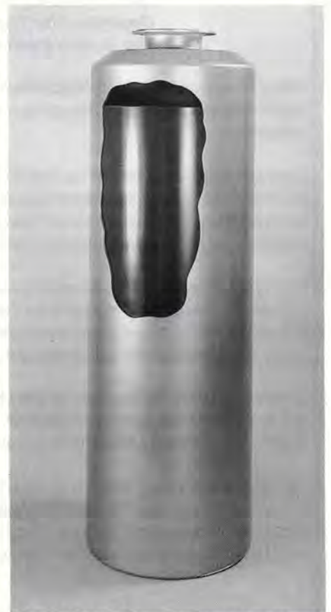
Model of a vitrified waste container, sectioned to show the waste inside.
