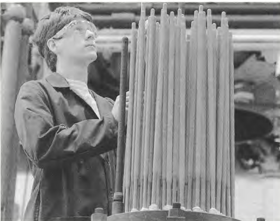
Assembler unloads newly coated tubular cells from the electrochemical vapour machine at the Westinghouse Electric Corporation's solid-oxide fuel cell pre-pilot manufacturing facility.
