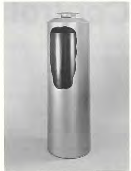
Model of a vitrified waste container, sectioned to show the glassified waste inside.
