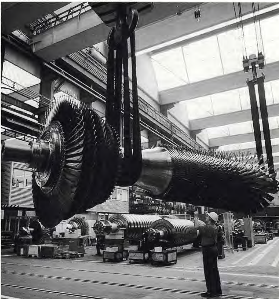
Bladed rotor of the GT13E2 gas turbine, with welded, maintenance-free rotor.
