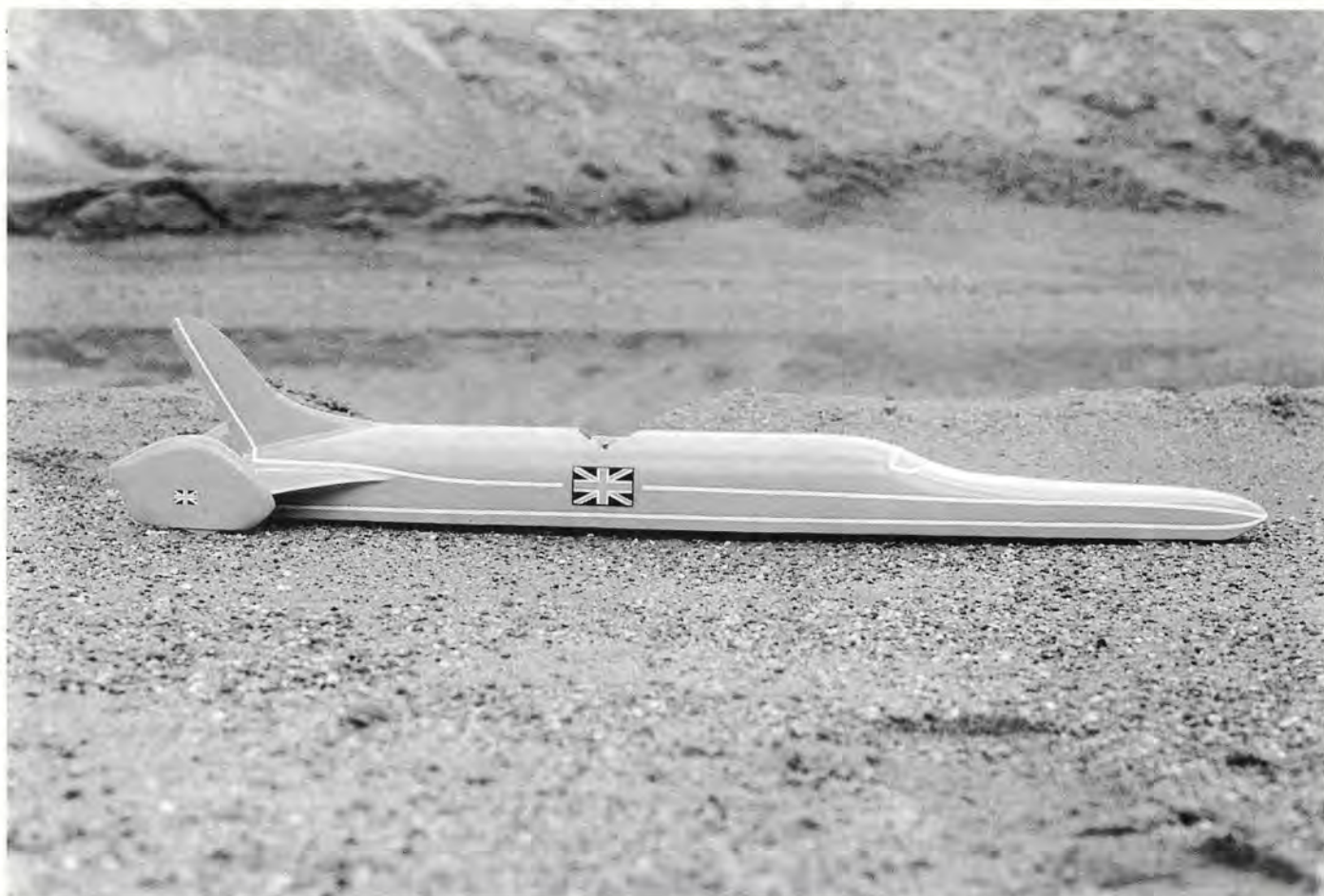
A 1/17th scale wind tunnel model of First Extreme International's diesel-powered Seven Tenths land speed record vehicle
