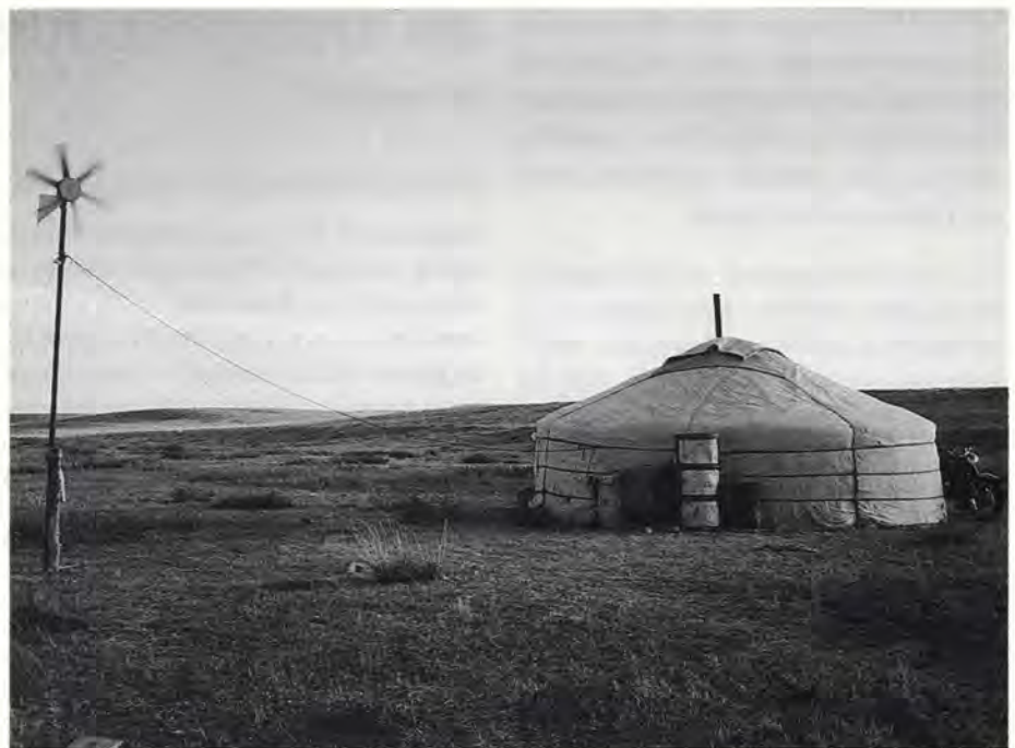
A 50 W battery charging wind-generator manufactured in Mongolia by the UK-Mongolian joint venture Monmar (UK partner: Marlec Ltd of Corby).
