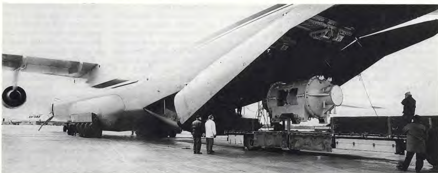
A recent airlift from Stockholm's Arlanda International Airport in Sweden of a 82.3 tonne aircooled turbogenerator unit. The unit was delivered to a papermill in Louisiana, USA.
