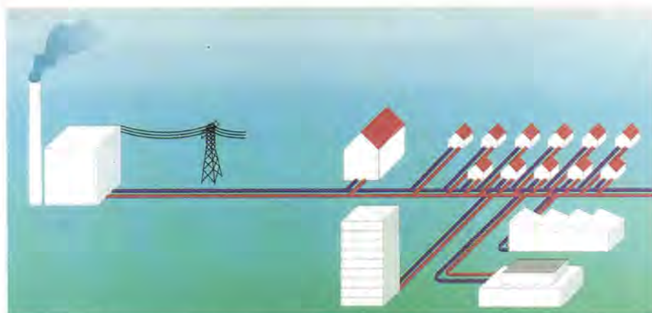
Community heating network: heat supplied to different buildings from a central source.
