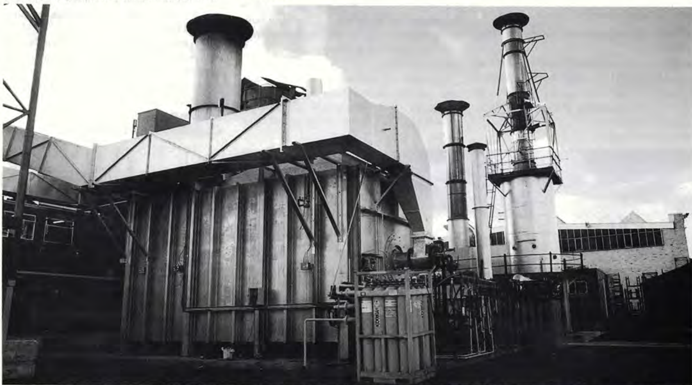
Test furnaces numbers one and four. Number one has an Enviromix Flat Flame 2000-140 natural draft gas burner with an output of 1MW. Furnace number four has a low NO x LNOG 3.57 dual fuel burner, with a fuel flow equivalent of 2MWth.
