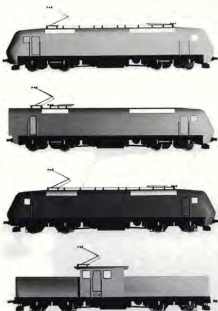
Eco2000 family of locomotives: at top a multipurpose locomotive with 6.4 MW drive rating; below it a power car; second from bottom, a freight train locomotive with two driver's cabs; at bottom a shunter. In principle all the types can be built with power ratings from 3 to 6.4 MW.
