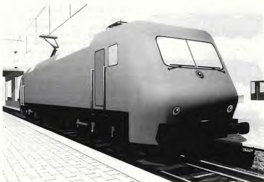
Standard design of the Eco2000 locomotive with its striking, virtually timeless appearance. Since it is made up of modules, customers can choose from various cab designs, or even create their own, unique cab front.
