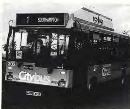
Southampton's natural gas Citybus, which carries its gas cylinders on the roof.
