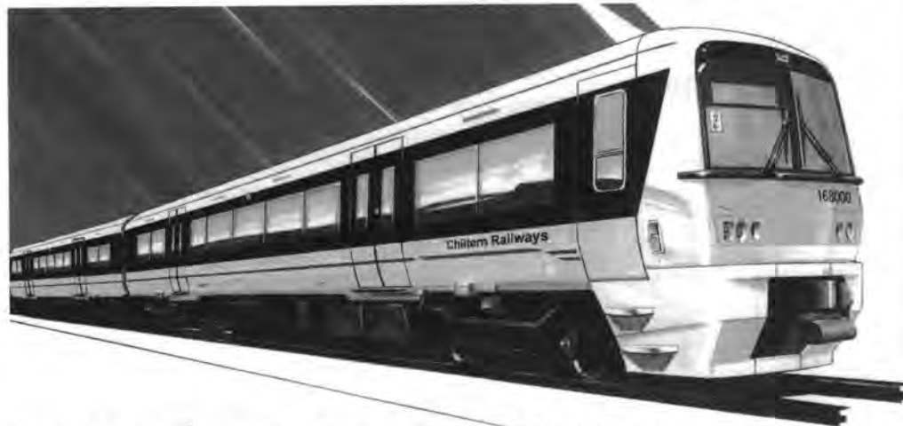
Chiltern Railways' new Class 168 Turbostar units will use Ni-Cd batteries
