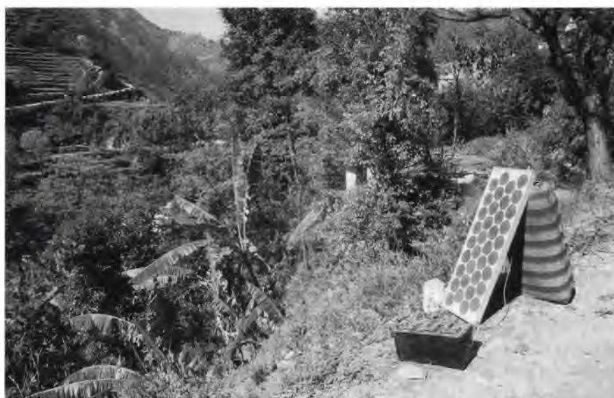
Photovoltaic module charging a lead-acid battery for use as a household lighting system in a remote Himalyan vilage in India. - Photo: IT Power
