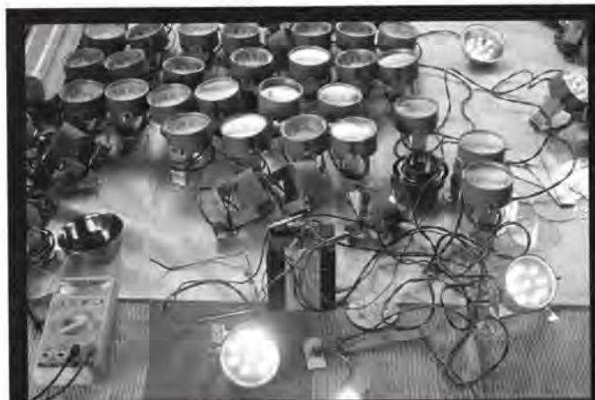
Some of the 0.1 W, white light-emitting diode (LED) lamps being supplied to villages in Nepal, India and Sri Lanka by Dave Irvine-Halliday's 'Light Up the World' Foundation based in Canada. Realising that a single such device can supply enough light for a child to read by, Irvine-Halliday founded his organisation to supply them where most needed. Using LED technology, the Foundation can light an entire village with less energy than that used by a single, incandescent 100 W light bulb. Irvine-Halliday has now become a '2002 Rolex Laureate' as a result.
