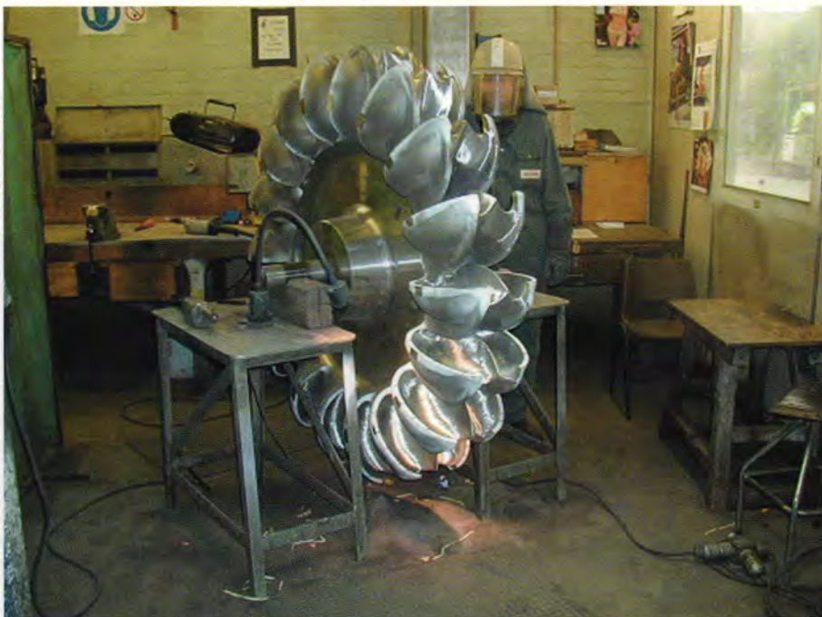
Fettling of the new 65 inch turbines at Gilkes' factory
