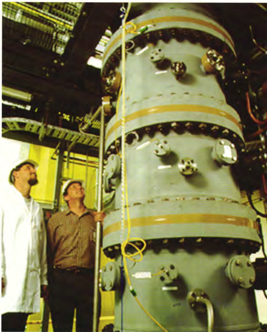
Coal gasifier being trialled in Queensland, Australia as part of work on integrated gasification combined cycle (IGCC) power generation.
