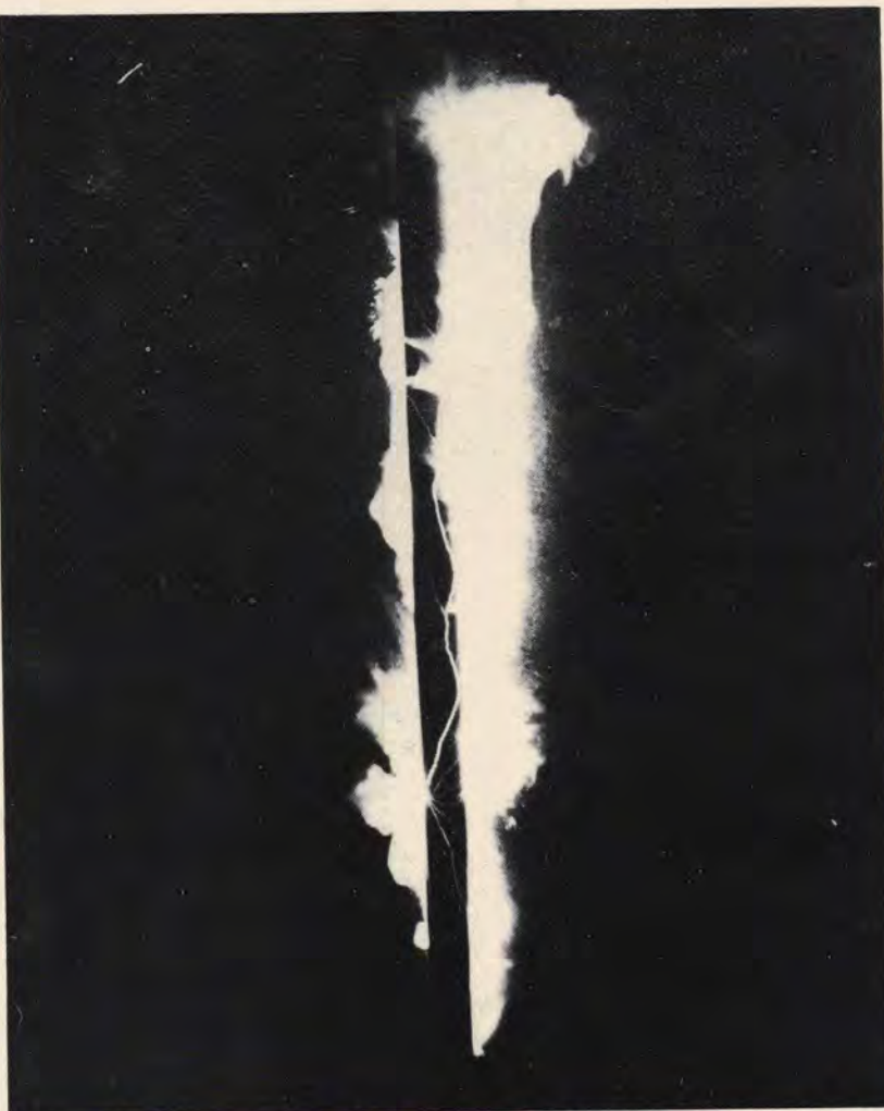
Electrostatic discharge cracking a plastic pipe conveying highly charged Diesel fuel. The lightning-type spark can be seen puncturing the pipe and igniting escaping fuel droplets.
