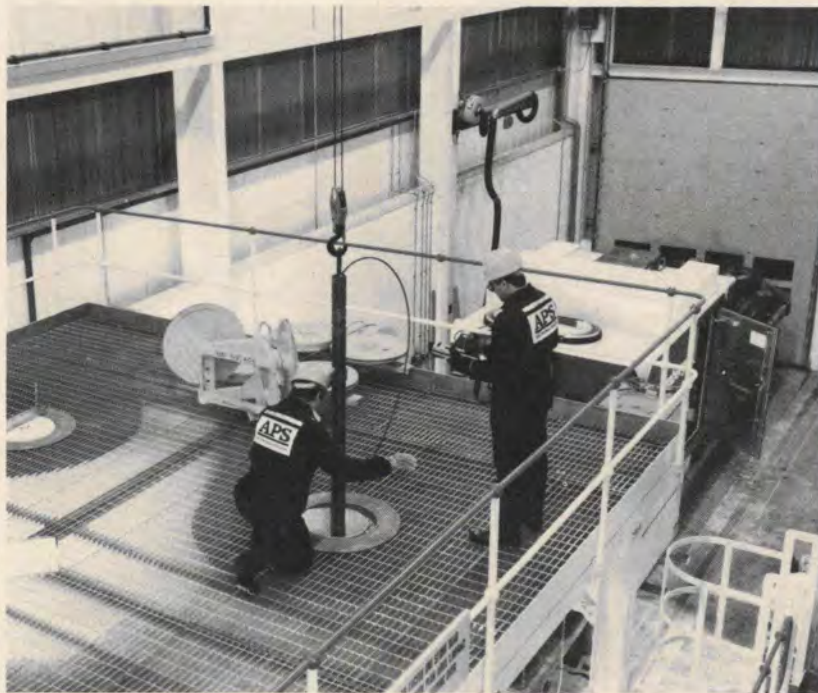
Testing a logging tool in a test pit.
