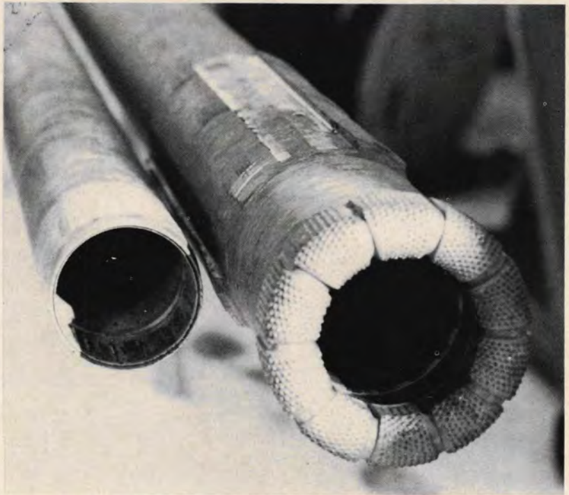
Slimhole core bit and inner barrel.
