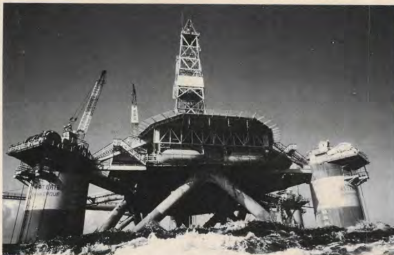
Forasol-operated semi-submersible rig Asterie which drilled in the Kudu gas field off Namibia.
