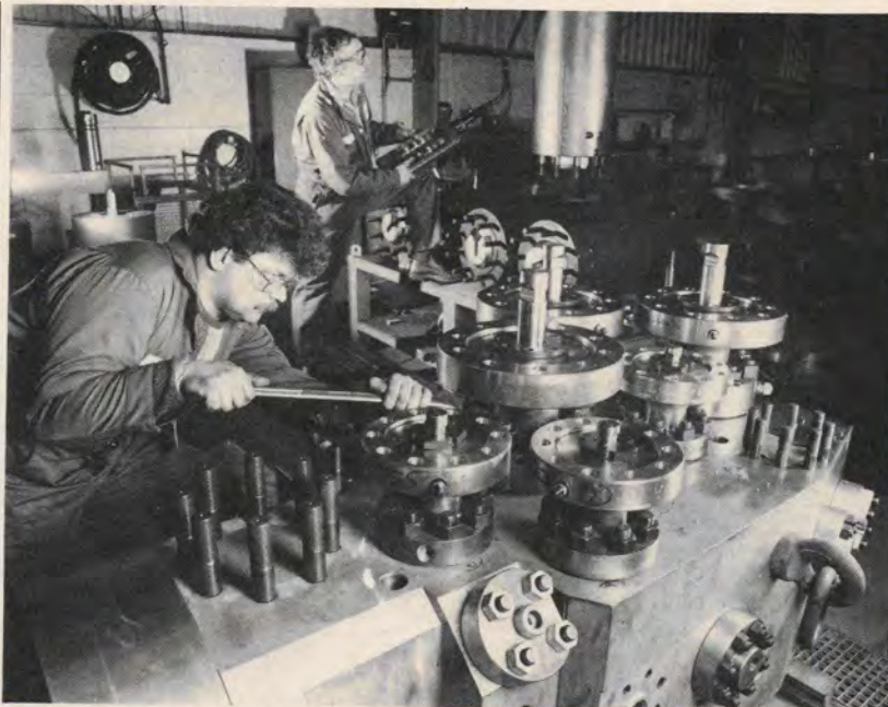
Assembly of part of the subsea valve for the Alwyn North Extension project, at the FMC factory, Dunfermline.
