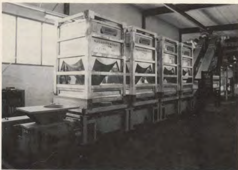
A clean and safe work environment and fast mixing are benefits claimed for an automated closed system for dosing drilling-mud additives, designed by Procon Engineering of Asker, Norway.
