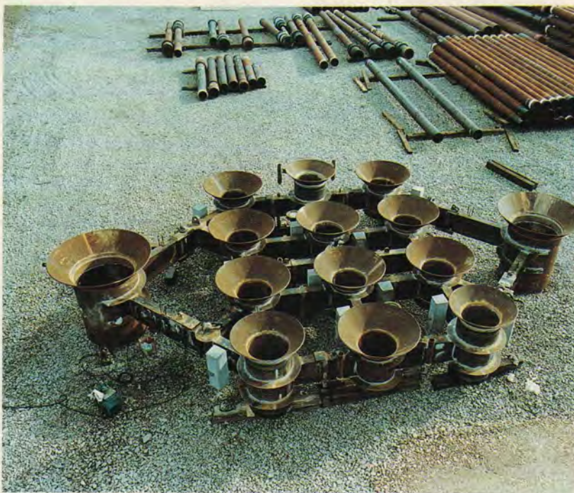
The sea-bed template for the Judy field before being taken offshore.
