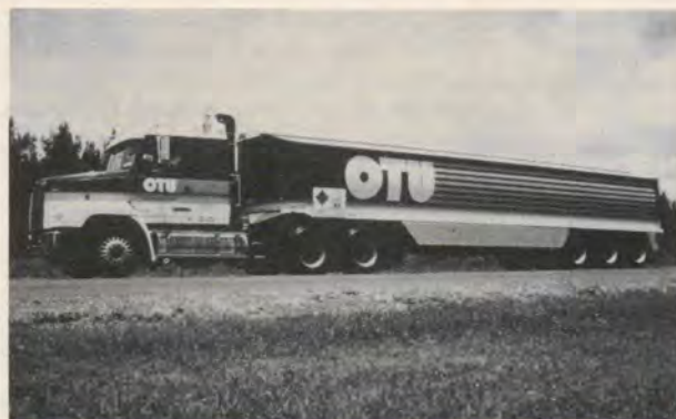
45,000 litre version of the 'THOMAS' tank in the livery of Australian haulier Universal Transport Operations.
