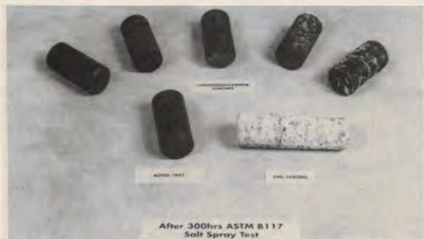
The comparison between Rocol 1PX1 durable barrier coating against other coatings after 300 hrs ASTM B117 Salt Spray Test.
