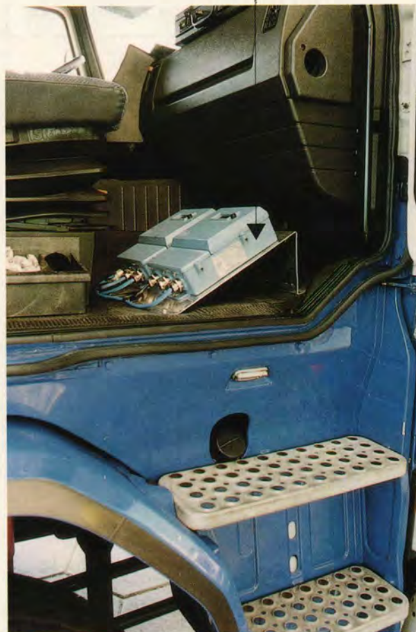
Plate A Readout units for Coriolis meter mounted in cab of LPG truck
