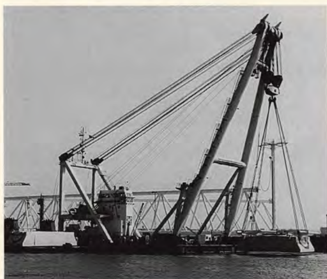
Smit Maritime Contractors has won a major heavy lift contract from Hibernia Management and Development Co for an offshore production platform currently being built in Newfoundland. A 1,200-tonne lift capacity Sheerlegs crane will carry out the work, using a 500-tonne capacity long boom. This offers a lifting height of 160m and a 100m reach.
