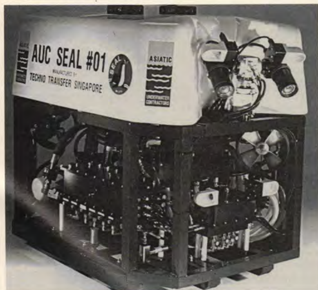
An advanced new light work class ROV
