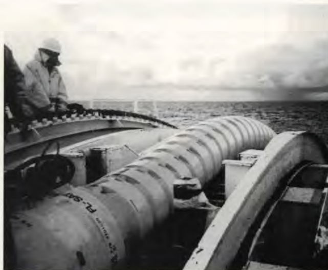
The pipeline bending restrictor at work on the Lulihua 11-1 development
