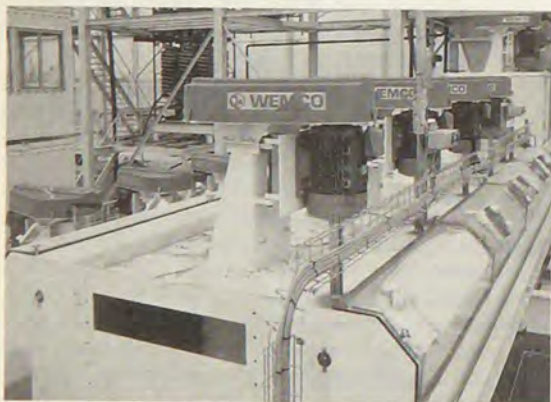
Soil cleaning in flotation unit.
