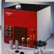
Below - Refrigerated Bath for Cloud and Pourpoint & Cold Filter Plugging Point conforming to IP and ASTM Methods.
