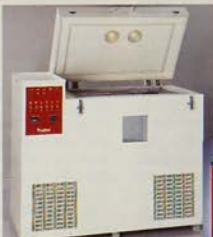
Above - Brookfield Viscometry Air Bath for preparation of Samples for Viscosity tests to ASTM D 2983.
