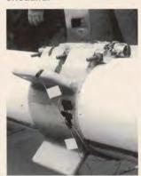
Clamp mounted on a section of riser undergoes tests
