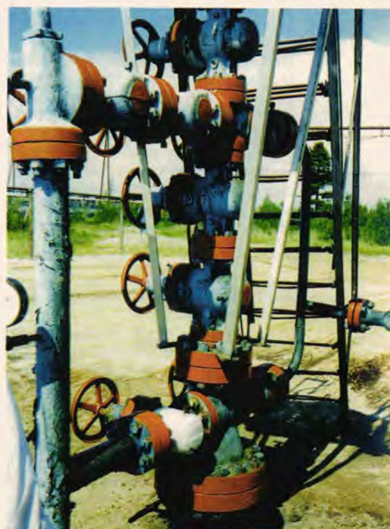
Typical western Siberian wellhead. Note the absence of a blow-out preventer (BOP) typical of operations in the region.
