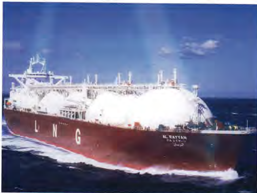
Delivered by Kawasaki Heavy Industries in March 1997, the 137,400 cm Al Rayyan is in service carrying LNG from Qatar to Japan as part of the Qatargas project
