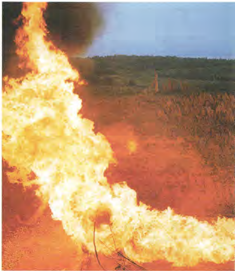
Small-scale jet fire testing at small scale at HSL, Buxton
