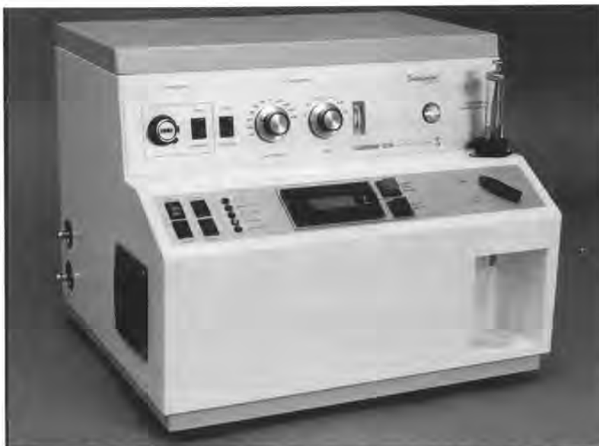
The UK Ministry of Defence, IATA and ASTM have now approved ASTM D 4305 (IP 422) Setapoint detector for automatic testing of the freeze point of aviation turbine fuels
