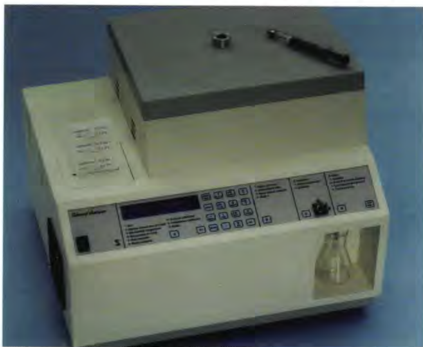
The Setavap analyser carries out automatic vapour pressure tests of gasoline in conformance with ASTM D 1591 (prEN 13016-1) and elevated temperatures (prEN 13016-2), as well as performing vapour liquid ratio tests to ASTM D 1588
