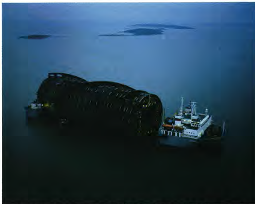
One half of the 225-metre long cylindrical hull for the Genesis field Spar, en-route from Finland to the Gulf of Mexico.
