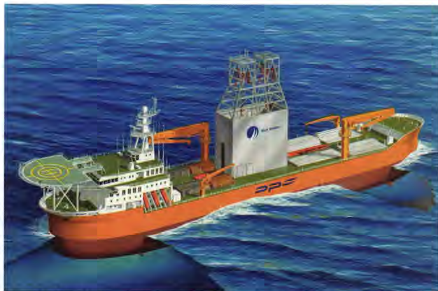
DPS 210, Aker Maritime's concept for combining floating drilling and production operations in deep water.
