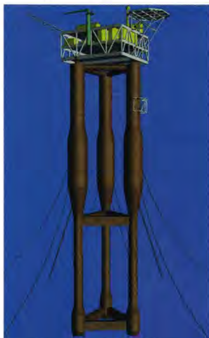
Kvaerner's deep draft floater will be capable of operating in waters between 130 metres and 2000 metres deep.
