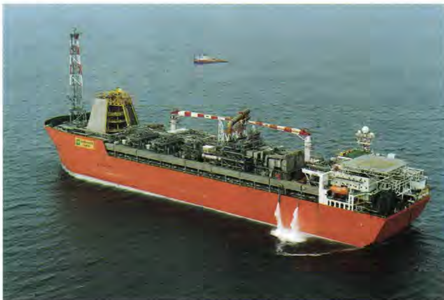
The Schiehallion FPSO is capable of handling 154,000 b/d of oil
