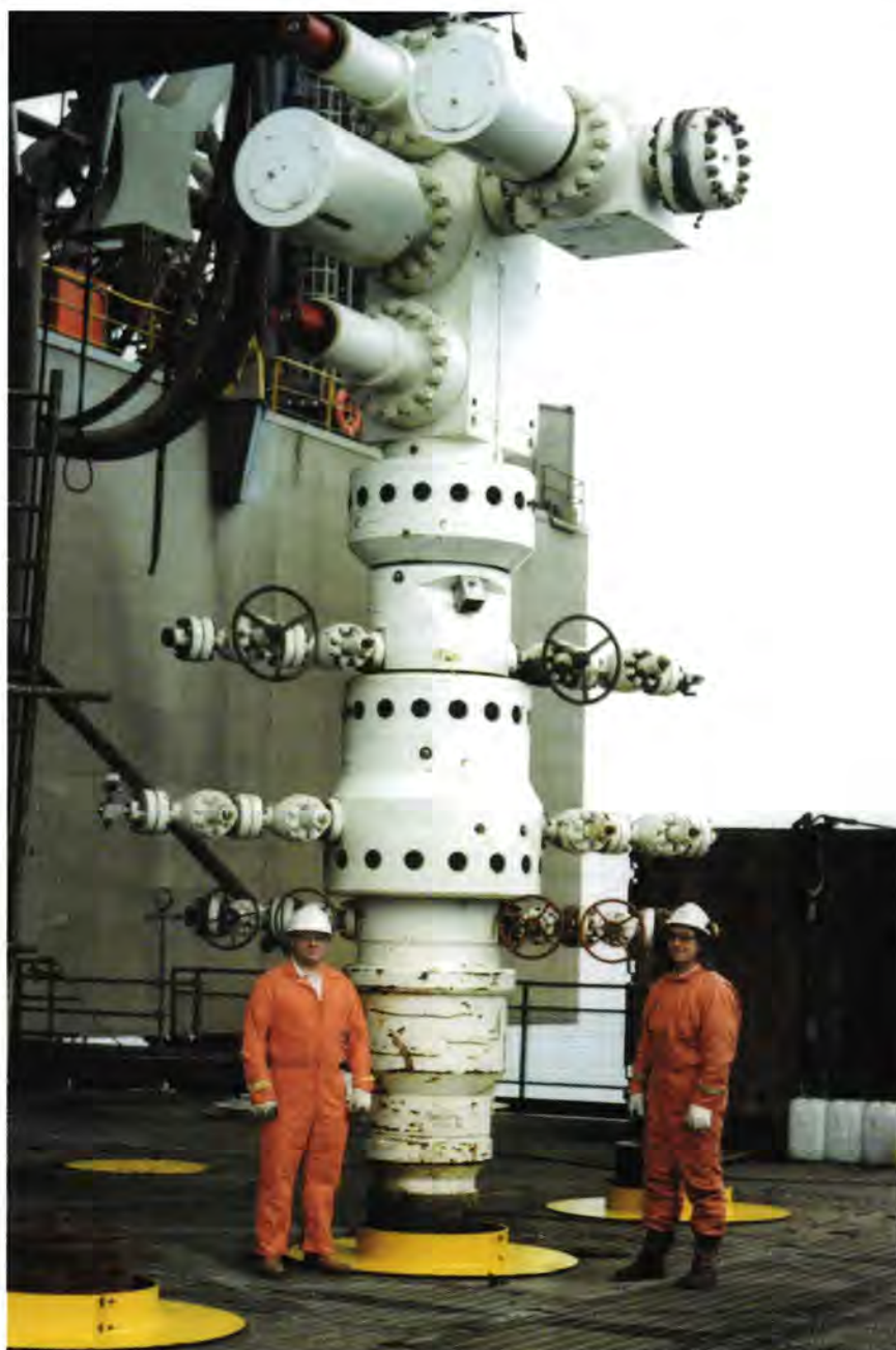
Shearwater will use what is claimed to be the world's first 15,000 psi xmas tree. The tree was installed in April 1998.
