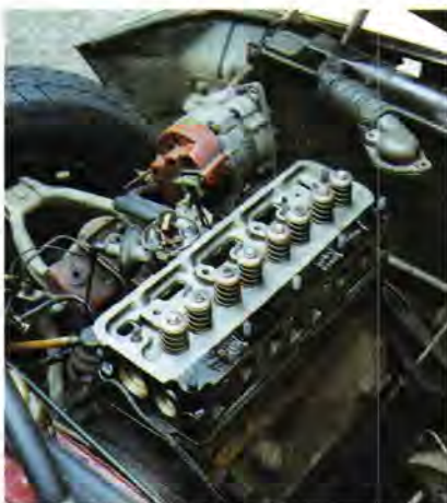
Converting the engine by fitting hardened valve seat inserts is the most expensive of the alternative options
