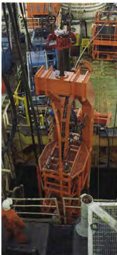
Coiled tubing extension frame suspended in derrick
