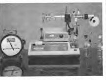
GRS2000 titrator (centre), GM2000 gas flow meter (left) and VA2000 moisture vaporiser (top)
