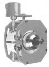
energised inner seal to stop the egress of the pipeline contents, plus a second selfenergised seal to prevent ingress of water from around the connector. The external seal allows the connector to work in deep waters of over 3,000 metres.
