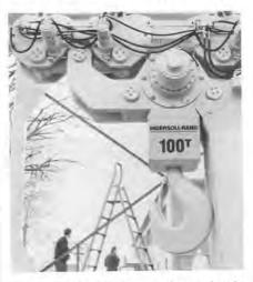
Ingersoll-Rand claims to have developed the world's most powerful hydraulic chain hoist system – capable of lifting up to 400 tonnes. The first unit to be built will be used for blow out preventer (BOP) handling applications on a new drilling platform currently being built by one of the world's largest drilling contractors.
