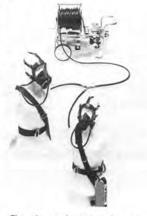
The air supply system has been designed so that air can be provided from a single cylinder and then switched to a second cylinder when the first is removed and replaced by a new cylinder, thereby providing continuous supply for extended durations, explains the company. In addition, the unit can be used in conjuction with a factory airline or compressor as a supplementary supply source.
