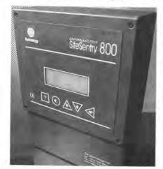
onscreen help and eight inputs monitoring any 4-20m signal, gives users maximum set-up choice, states the company.
