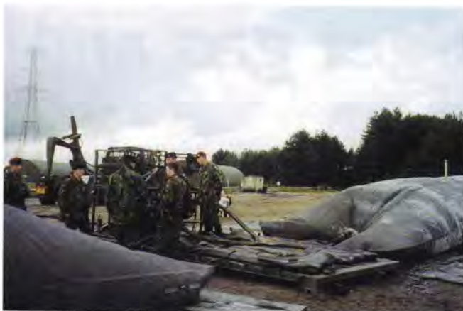
Figures 3a and 3b: The Donaldson Flatrack fuelling package with pump (left of photo) and filter water separator (right)
