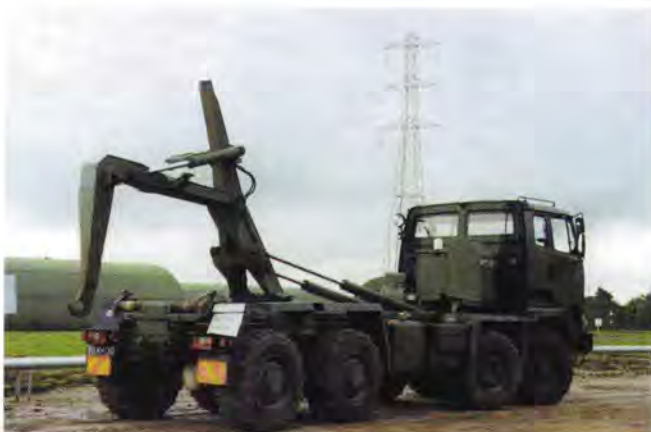
Figure 4: The Donaldson Flatrack system can be carried by a dismountable rack off-loading and pick-up system (DROPE) vehicle.
