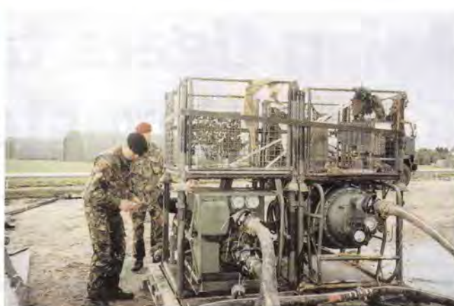
Figures 3a and 3b: The Donaldson Flatrack fuelling package with pump (left of photo) and filter water separator (right)
