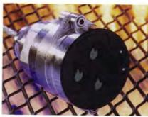
The second-generation Det-Tronics X3300 infrared optical flame detector is designed to sense the smallest fires in process or production facilities, indoor and outdoor plants, oil refineries and offshore platforms. For example, it can sense a 0.1m² gasoline fire at distances over 60 metres, states the manufacturer.
