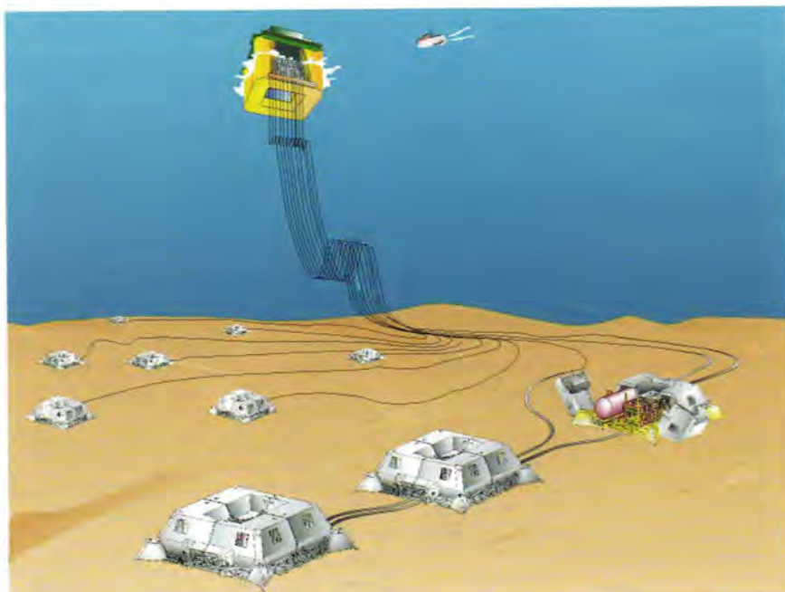
Figure 1: The world's first subsea separation and injection system, Subsis, will soon be operating in Norsk Hydro's Troll field
