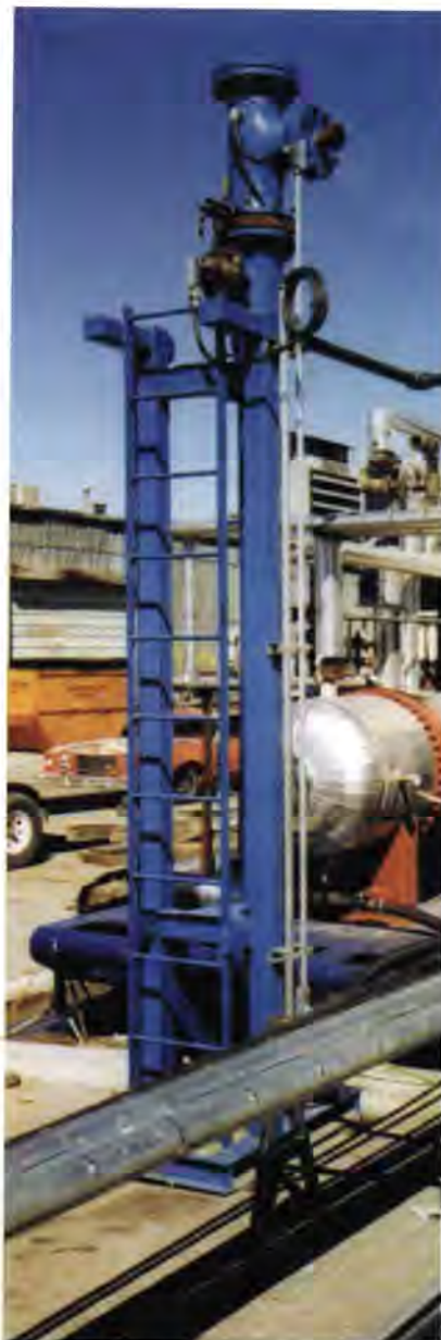
Kvaerner's compact coalescer under test
