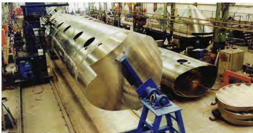
Tank sections are continuously welded by machine for consistency
