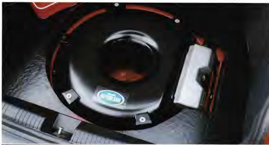
An LPG tank in the spare wheel space
